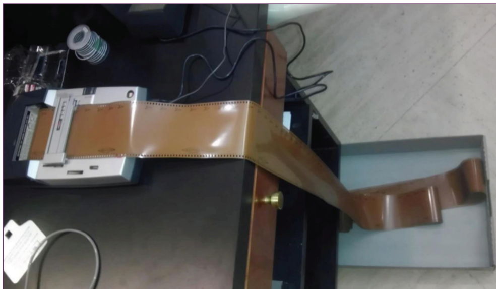
Image 1. The above photo shows the working Rols audio player that we purchased with one of the Rols dictation tapes loaded into it. The device was designed without a take-up reel so the audiotape just spools off onto the floor as it plays or records. 154
