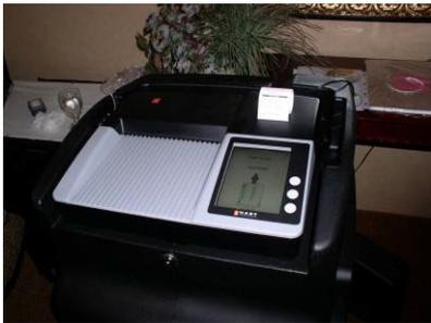
The eScan is a precinct based paper ballot digital scanner (upper picture on the left). Voters insert their ballots into the eScan unit. It digitally scans the ballots, storing a CVR in a MBB, and feeds the ballots into the ballot box (lower picture to the left) which serves as the base for the unit. It is configured to reject ballots with over voted contests and ballots which are blank. The eScan
