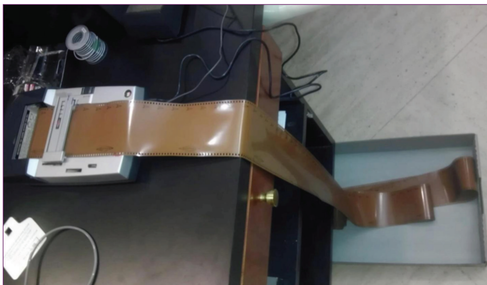
Image 1. The above photo shows the working Rols audio player that we purchased with one of the Rols dictation tapes loaded onto it. The device was designed without a take-up reel so the audiotape just spools off onto the floor as it plays or records. 154
