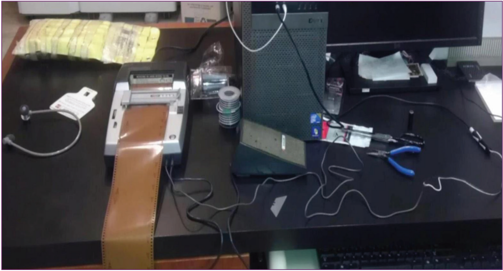
Image 3. The above photo shows from left to right: headphones without the cable attached; Rols audio player; audio wire and its packaging; computer; and in front of that is the foot pedal used to both play the Rols audio and rewind it depending on the amount of pressure applied to the pedal. The thicker dark cable coming off of the Rols audio player goes to the foot pedal and the smaller one usually attaches to the headphones (far left) but was removed to allow staff to attach wire leads to the new headphone adapter. Finally, an audio line hooks into the new headphone adapter and plugs into the front of the computer (black cable). 161
