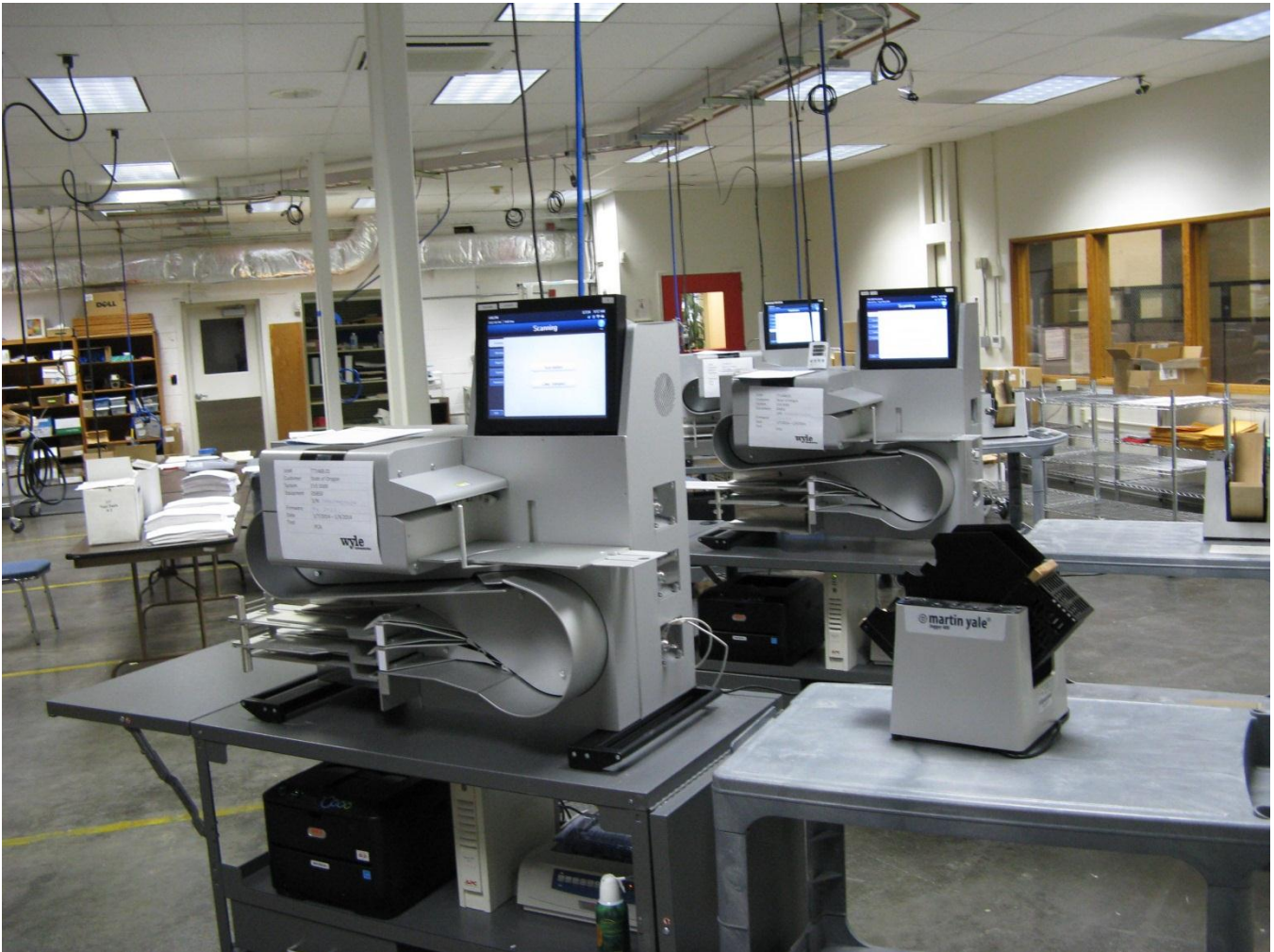
Photograph 12: DS850 Testing Setup
